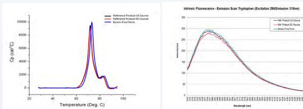
Figure 2: DSC profile of the Final ONS formulation overlay with Reference Product, note the  $T_m$  being slightly increased
